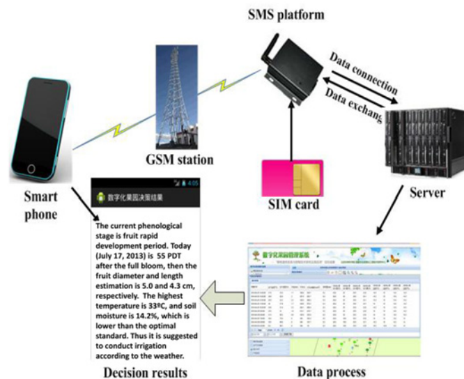
Fig 5. Schematic showing the use of digital orchard management information system.
