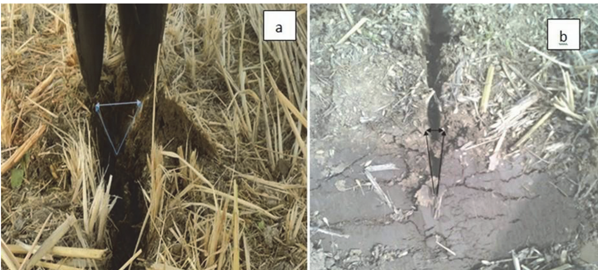
Fig 8. (a) Furrow profile of DD450 (b) Furrow profile of DD330.
