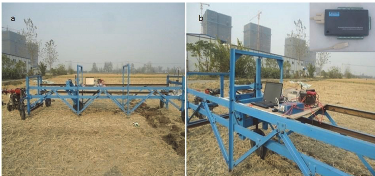
Fig 2. (a) Test bench with power source (b) Data acquisition system with data acquisition card.
