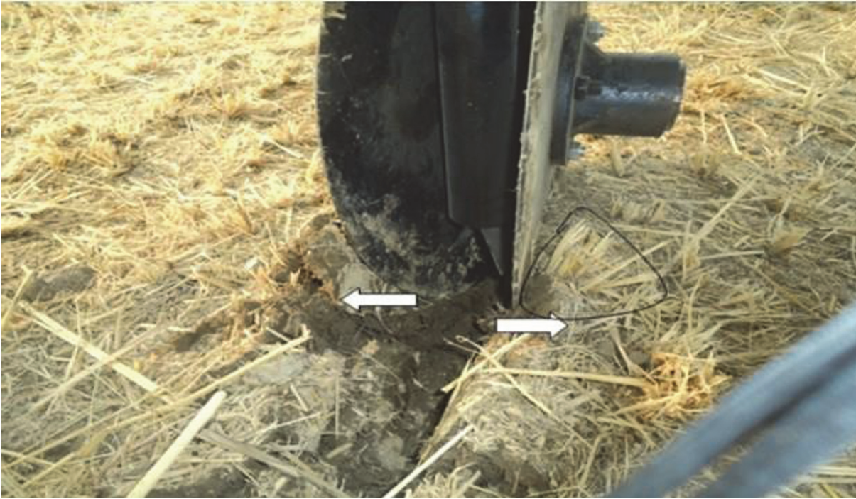
Fig 7. Soil movement and furrow opening mechanism by double disc opener.
