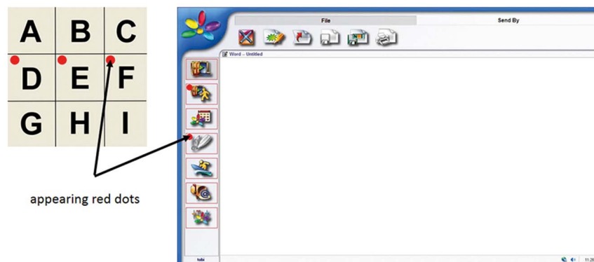
Figure 1. Transfer of the matrix based speller paradigm to the Qualilife software. Left: To adapt end-users to the flashing of dots, those were placed in each cell of the well familiar matrix. Instead of the letters those dots were flashed. Right: Screen shot of the Qualilife communication application. The now familiar red dots were assigned to each option of the Qualilife communication and control surface. Red dots appear randomly at each possible “button” to press. Attention needs to be focused on the specific button to be pressed by counting how often the red dot is appearing.
