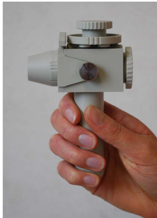
Figure 1. The test inhaler with exchangeable airflow resistance (disk on top) and the conical mouthpiece.
