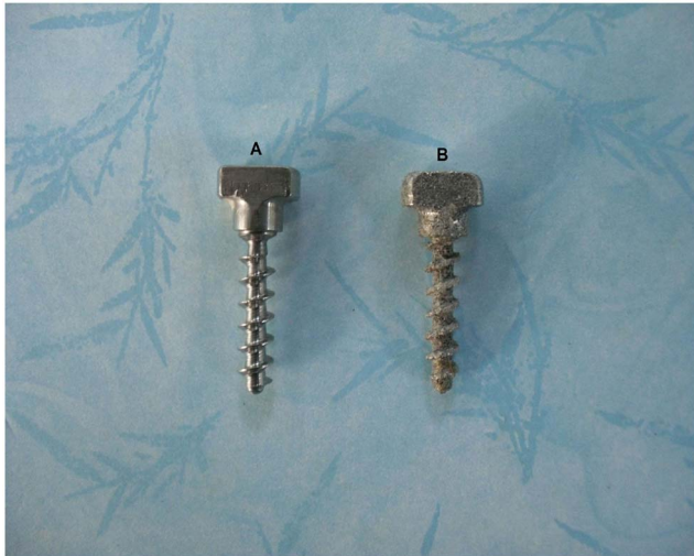
Figure 1. (A) Conventional titanium alloy screw with a smooth surface (SS). (B) Titanium alloy screws with a roughened surface (RS) were fabricated by electron beam melting (EBM). doi:10.1371/journal.pone.0096179.g001
