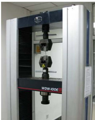
Figure 1. Photo of the universal tester used for tensile test. doi:10.1371/journal.pone.0093066.g001
