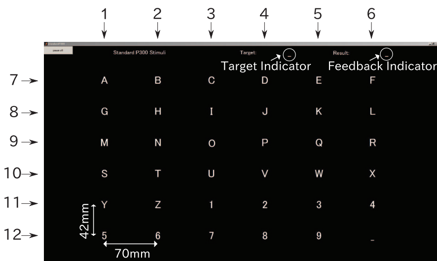
Figure 3. Stimulator for the P300-based BCI. It has 36 gray letters that form a matrix in the center. Each column of the matrix is numbered 1–6 and each row 7–12. A target letter is provided at the top center of the stimulator and the predicted letter is shown at the top right as feedback in test sessions. doi:10.1371/journal.pone.0093045.g003
