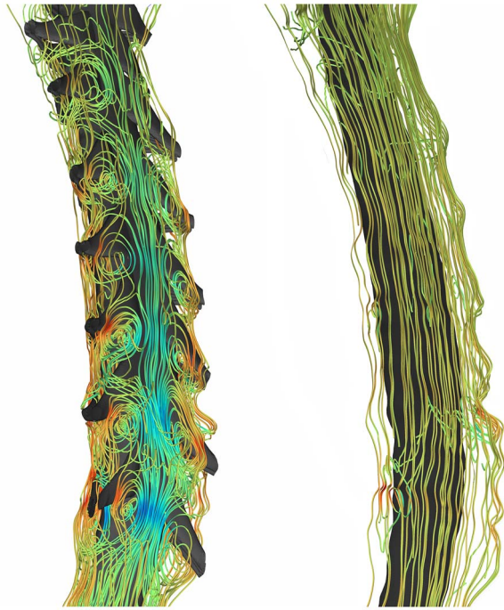
Figure 7. Streamline plots for healthy case with fine structures (left) and without fine structures (right). Streamlines are calculated at t = 0.56 s. doi:10.1371/journal.pone.0091888.g007
