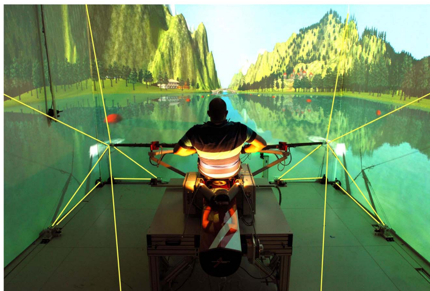
Figure 1. Training in the scull rowing simulator of the SMS-Lab at ETH Zurich. This scull rowing simulator is set up in a CAVE comprising auditory-, visual-, and haptic displays. doi:10.1371/journal.pone.0082145.g001
