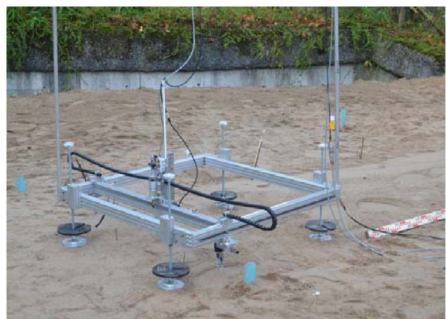
Figure 2. 3D laser scanner developed and custom-built for recording animal tracks. The scanner covers an area of 800×800 mm.
