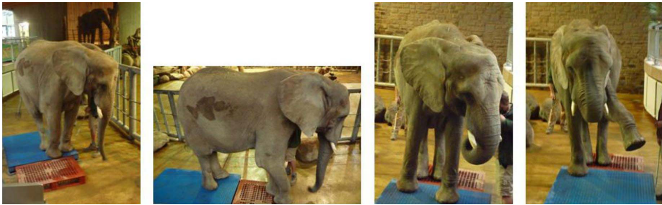
Figure 8. Weighing the elephant cow Sweeny. The following loads were measured: a) the elephant was standing with all limbs on the scale ( m = 2530 kg), b) the load carried by both hindlimbs ( m = 1125 kg), c) the load carried by both forelimbs ( m = 1530 kg), and d) the load carried by one forelimb ( m = 1390 kg). doi:10.1371/journal.pone.0077606.g008
