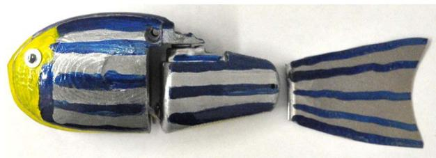
**Figure 1. Robotic fish used in our experiments.** The color pattern, aspect ratio, and shape of the caudal fin of the mobile robotic fish used in our experiments matched that of a zebrafish. doi:10.1371/journal.pone.0076123.g001
