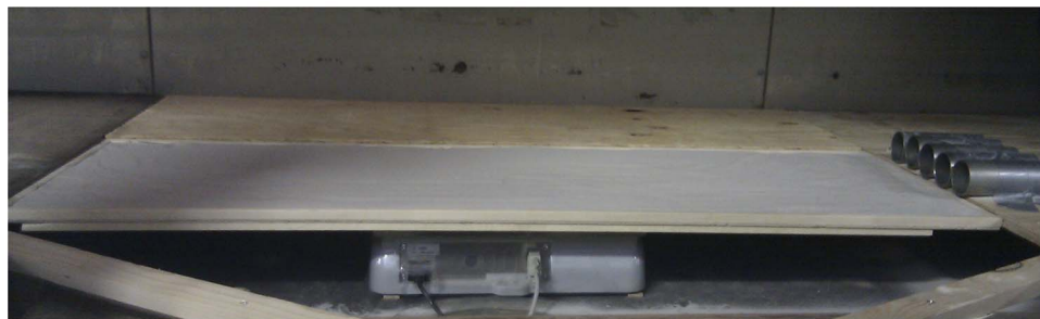
Figure 3. Image of the experimental setup. The balance was placed underneath the test tray in order to measure the weight of the sediment throughout the experiment. The image taken during the calibration, when the five saltiphones were placed next to each other. doi:10.1371/journal.pone.0074007.g003
