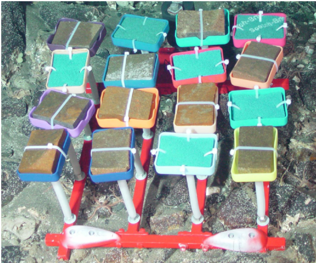
Figure 2. Array of larval settlement collectors at deployment in 2006 (South wall: 671 m). Collectors included either a basalt rock ( \sim 7 \times 10 \times 2 cm) supported by a plastic ring ( n = 10 ), or mesh pads ( \sim 7.5 \times 10 \times 1.5 cm, blue 'Scotch-Brite' pads, mesh openings: \sim 3.5 mm 2 ) ( n = 6 ). doi:10.1371/journal.pone.0065394.g002
