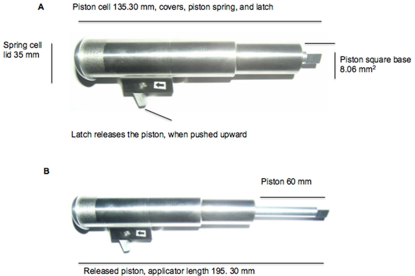
Figure 1. Illustration of the metal applicator used for the MN applications. (A) A digital photograph of the applicator prior to release of the piston. (B) A digital photograph of the applicator after the release of the piston. The digital images were captured using an Olympus C5060 WZ digital camera (Olympus Corporation, Lake Success, NY, USA) and were edited with Adobe® Photoshop® CS5 (Extended Version 12.0×64, Adobe Systems Inc., San Jose, CA, USA).
