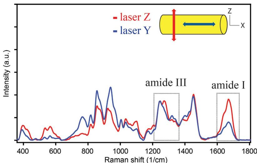
**Figure 1. Polarized Raman spectroscopy of RTT.** Spectra taken at the same spot of the sample were collected with two different laser polarization orientations [parallel (laser X, blue line) and perpendicular (laser Z, red line) to the tendon axis]. A large anisotropy of the amide I band in the two different laser to fiber configurations is due to the preferential orientation of vibrational units along the main axis of the tendon. doi:10.1371/journal.pone.0063518.g001
