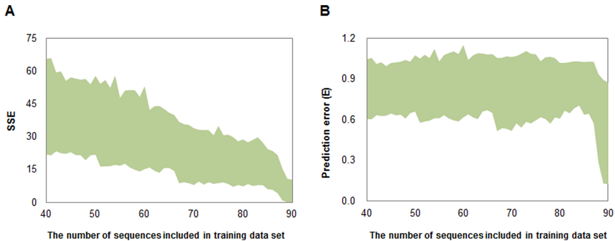
Figure 2. Functional relationship between the prediction performance of ANN models and the scale of training data set. Training data set scale ranges from 40 to 90 sequences. (A) Maximum and minimum SSE values of prediction as a function of training data set scale. (B) Maximum and minimum prediction errors as a function of training data set scale. doi:10.1371/journal.pone.0060288.g002
