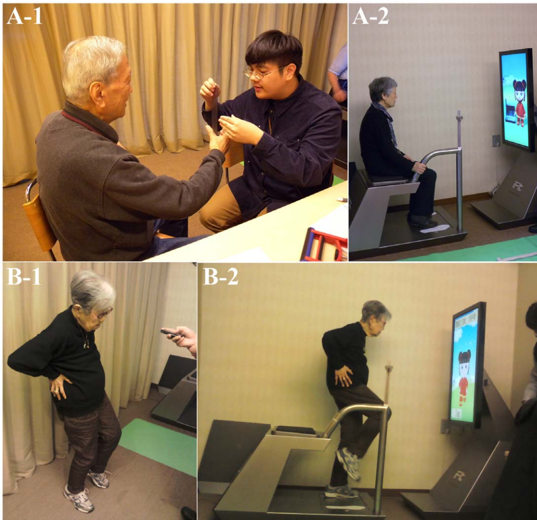
Figure 3. The experimental procedures for the traditional and iFit tests. (A-1) The conventional reaction-time measurement. (A-2) The iFit reaction-time measurement. (B-1) The conventional balance measurement. (B-2) The iFit balance measurement. doi:10.1371/journal.pone.0057452.g003
