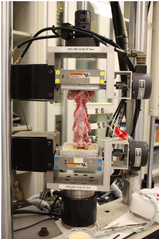
Figure 5. Biomechanical testing of ACVC implanted C1–C5 segments using a MTS machine. doi:10.1371/journal.pone.0052910.g005
