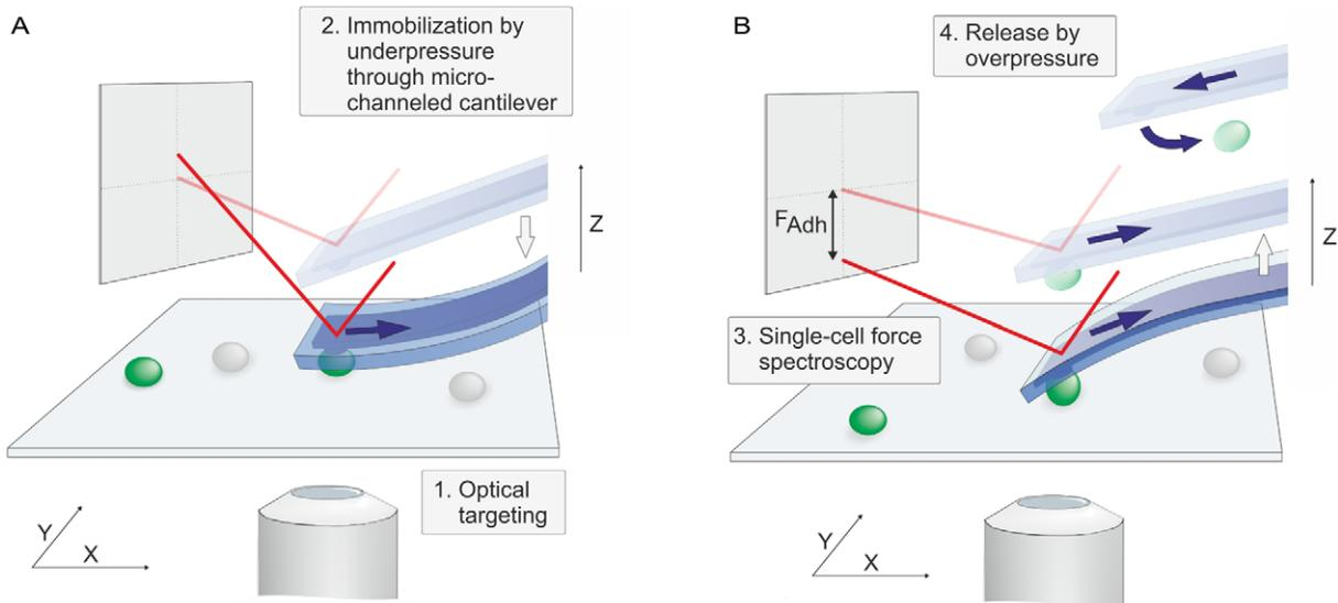
**Figure 1. FluidFM-based single-cell force spectroscopy.** Schematic view of the experimental principle. (A) Cell targeting and immobilization to the cantilever through the application of under pressure. (B) Single-cell force spectroscopy and subsequent release of the measured cell. doi:10.1371/journal.pone.0052712.g001
