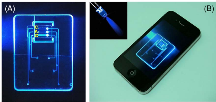
Figure 5. End-point detection of An. gambiae DNA recorded with iPhone 4. (A) An enlarged image of the illuminated chip. Reactor G emits visible light while reactors A and C stay dark. (B) Photograph of iPhone 4 with mosquito-on-a-chip fluorescence image. A minute, reusable, light-emitting diode (inset) excites the fluorescence emission. doi:10.1371/journal.pone.0042222.g005
