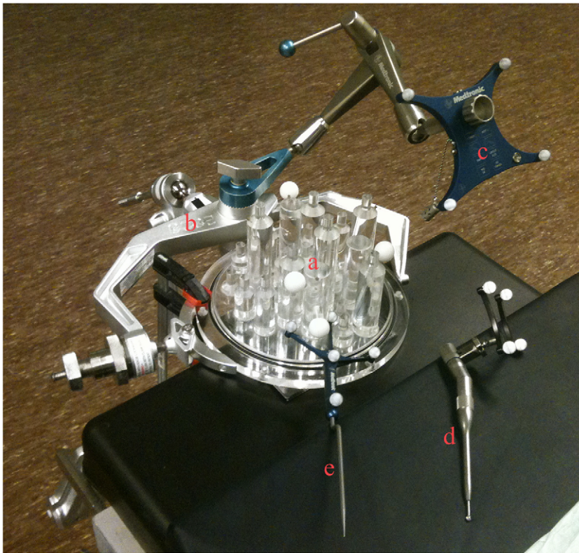
Figure 6. Drill Tracking Accuracy Experimental Setup. The setup in the operating room during drill tracking accuracy experiments on the cylinder and ball phantom (a) is shown. Note the head clamp (b) and reference frame (c). Registration of the phantom was performed via four rigidly attached screws that served as fiducial markers. The top of the cylinders were touched with the drill (d) with attached tracking frame and pointer (e) and the image coordinates were recorded and compared with the actual positions to yield target registration errors. doi:10.1371/journal.pone.0041262.g006
