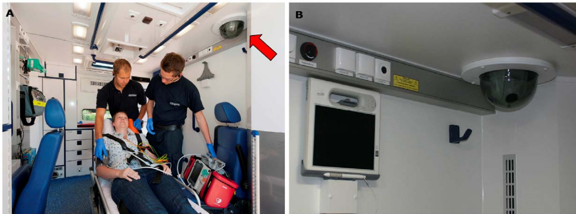
Figure 2. Interior of the telemedically equipped ambulance. Picture A. Trailing scene with a volunteer in the role of a patient and paramedics from the fire department. The video camera is behind a glass cover (Picture B and indicated by the red arrow). The camera position in the ceiling allows zooming to the patient's face and looking at all body regions from the teleconsultation center. Picture A provided by Peter Winandy, Aachen, Germany.
