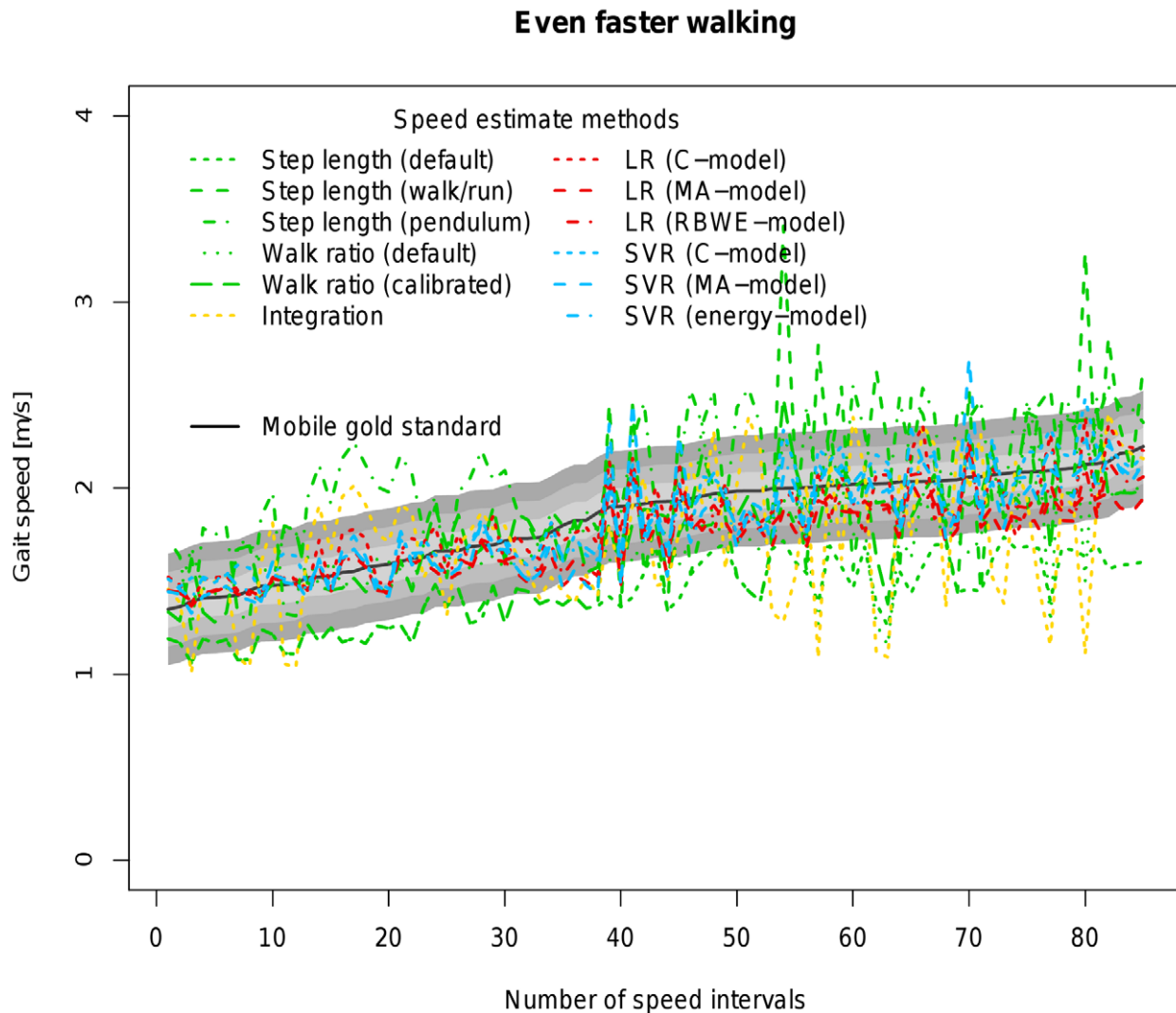
Figure 5. Visualization of coverage probability for even faster walking in the indoor ecological validation. The black solid line represents speed as measured by the mobile gold standard for even faster walking. Green, yellow, red and blue lines in different linestyles represent different speed estimates by different algorithms and models. The filled areas colored from light to dark grey around the black solid line indicate coverage probability levels from 0.1 to 0.3 m/s. Speed intervals are sorted increasingly across all participants for reasons of clarity and readability. doi:10.1371/journal.pone.0023080.g005
