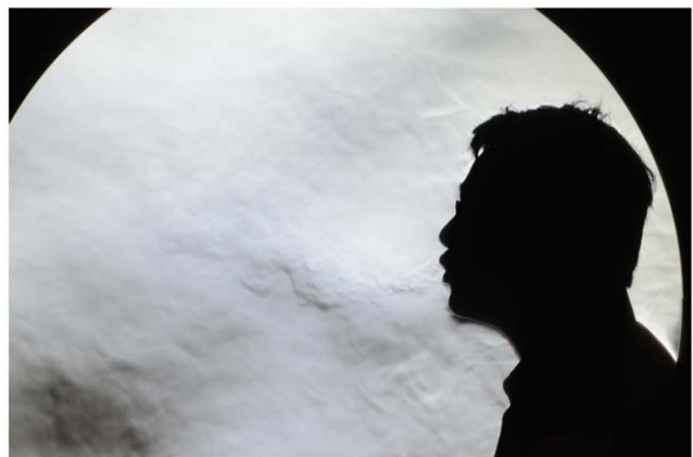
Figure 3. Typical position of a single subject in front of the schlieren mirror. The exhalation puffs can be seen as disturbances in the 'texture' in front of the head (images obtained using a Nikon D7000 SLR in HD 1920×1080 live video mode).
