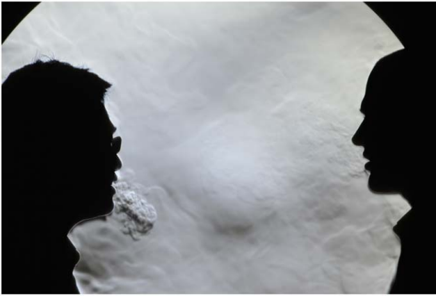
Figure 4. Two subjects in position in front of the schlieren mirror. For some experiments, two subjects may face each other across the mirror in order to visualize how their exhaled airflows interact during, e.g. during normal conversation (images obtained using a Nikon D7000 SLR in HD 1920×1080 live video mode). doi:10.1371/journal.pone.0021392.g004
