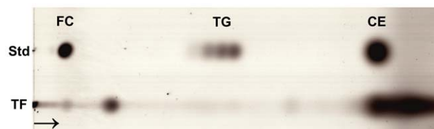
Figure 2. TLC of non-polar lipids. TF, tear fluid; Std, standard solution containing free cholesterol (FC), triglycerides (TG), and cholesteryl oleate (CE). The arrow shows the direction of the eluent flow.
