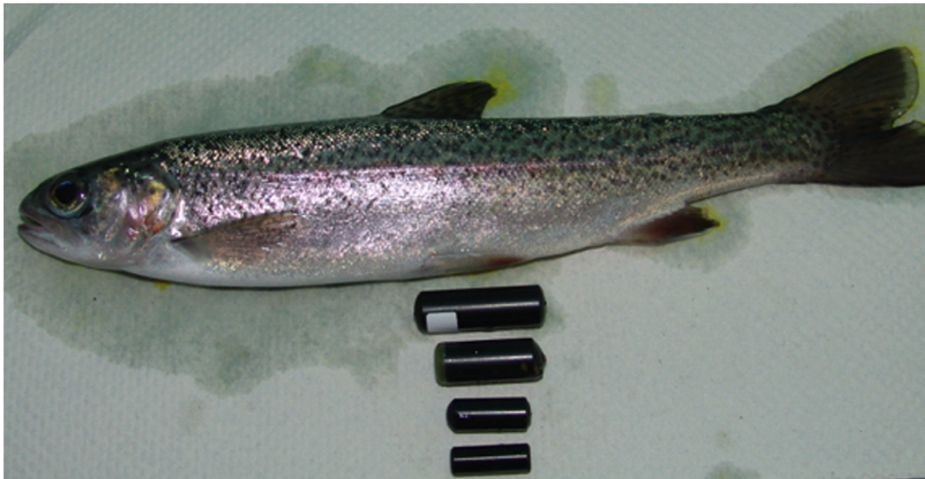
Figure 1. A salmon smolt shown with the variety of acoustic tags and how the size of acoustic tag has become reduced as the technology advanced.
