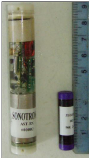
Figure 2. Animal-attached/implanted proximity detector. Example of the ARX acoustic receiver (left) and IBT transmitter (right) used in the study on lemon sharks. doi:10.1371/journal.pone.0009324.g002
