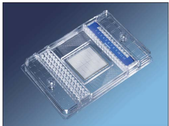
Figure 1. A digital array has 12 panels of 765 reaction chambers each. PCR mixes are loaded into each panel and single DNA molecules are randomly partitioned into the chambers. The digital array can be thermocycled, imaged on a BioMark instrument, and the data analyzed using the Digital PCR Analysis software. doi:10.1371/journal.pone.0002876.g001
