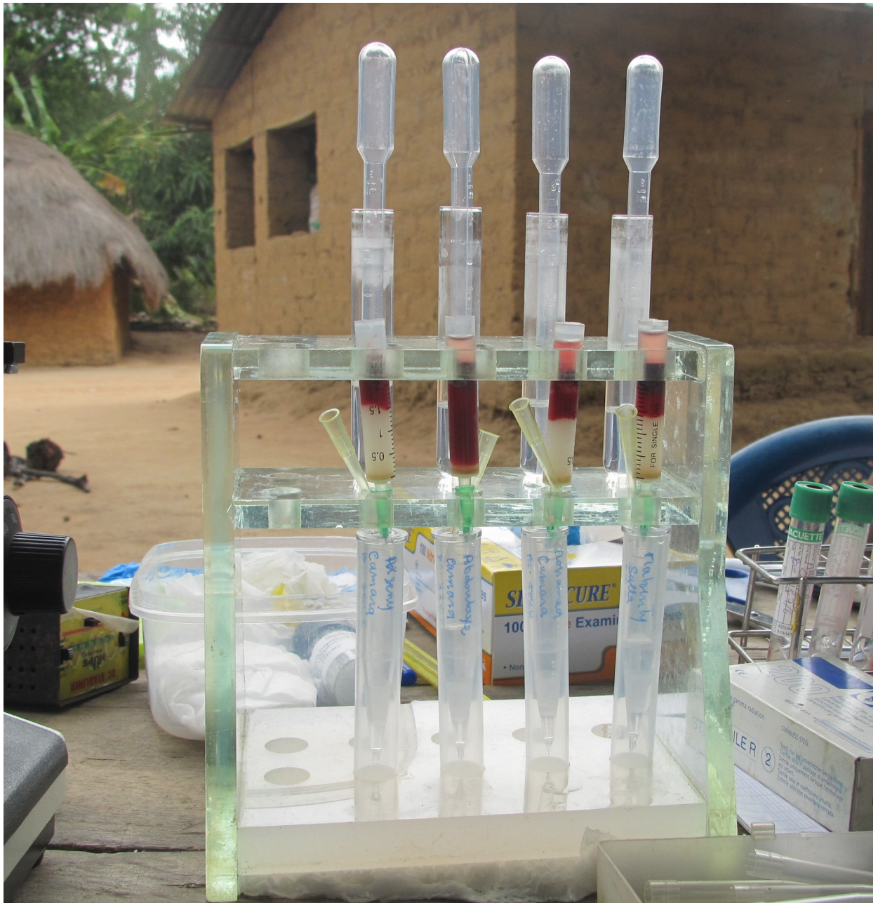
Fig 1. DEAE cellulose minicolumns for the diagnosis of HAT in CATT-positive suspects during mass screening. CATT, Card Agglutination Test for Trypanosomiasis; DEAE, di-ethyl amino ethyl; HAT, human African trypanosomiasis.
