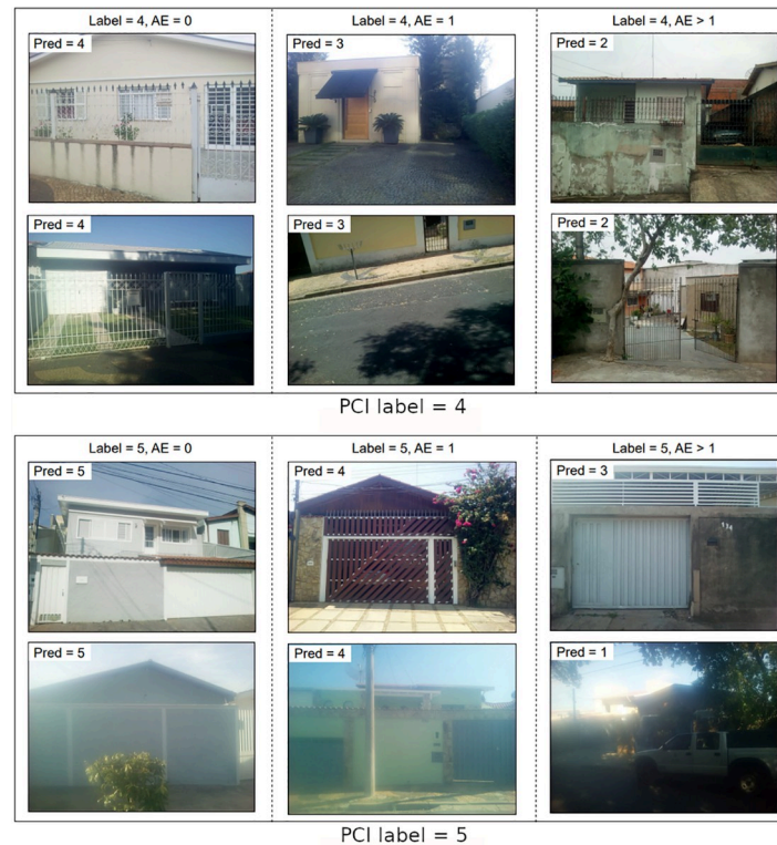
Fig 5. Random facade samples with different labels for facade conditions. Images are divided into three columns according to PCINet's ability to classify them, from left to right: correctly classified samples, wrongly classified samples with absolute error (AE) equal to 1, and wrongly classified samples with absolute error (AE) greater than 1.
