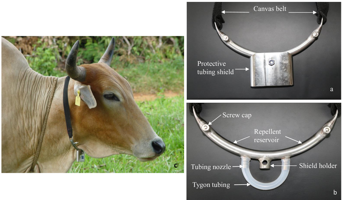
Fig 3. Repellent dispenser developed to deliver waterbuck repellent compounds for cattle. (a) Dispenser with protective shield and (b) without protective shield to show tubing from which the repellent compounds are released and (c) a cow with a repellent collar.
