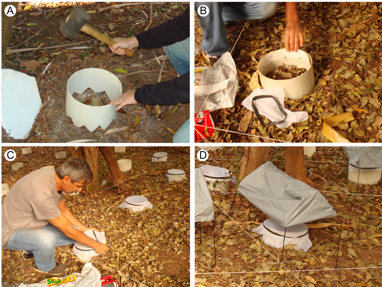
Figure 2. Emergence traps. A: Fixing emergence trap to the ground. The serrated bottom facilitates its fixation in the soil. B: Placing the adhesive paper. C: Covering the emergence trap with a sand fly-proof fine mesh to prevent sand flies escaping. D: Emergence traps covered with a small tent. doi:10.1371/journal.pntd.0002443.g002
