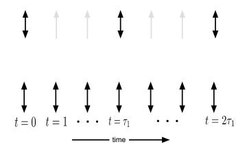
Figure 2. Timing of the input and output messages to Node k. The message passing between the node and its children occur at intervals of 1 time step, where as the message passing between the node and its parents occur at intervals of  $\tau_k$  time steps.
