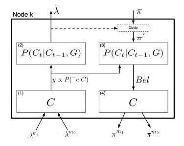
Figure 1. Block diagram of belief propagation computations in an HTM node.
