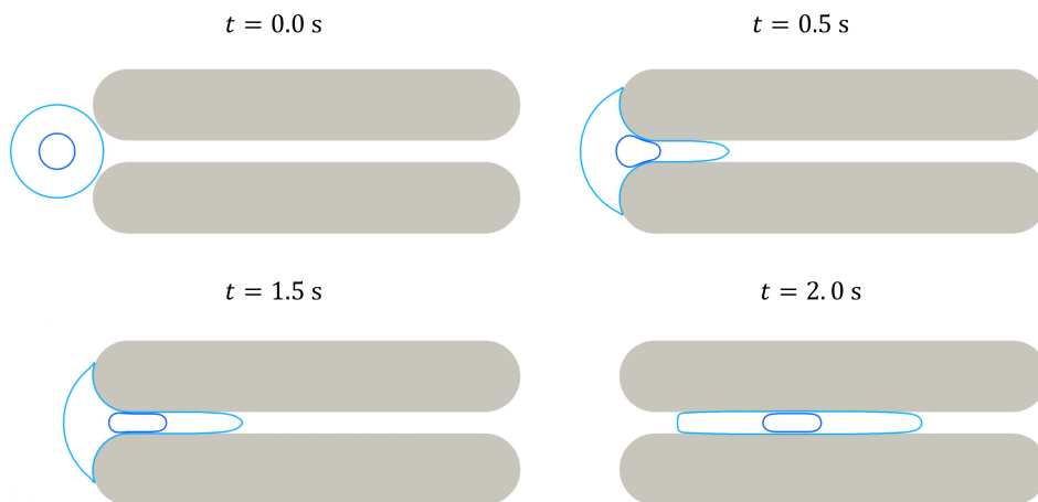
Fig 3. Snapshots of the cell plasma membrane (light blue closed curve) and the nuclear envelope (dark blue curve) at different time points for a microchannel width of 6 \mu\text{m} . The simulation was carried out using the parameter values reported in Table 1.
