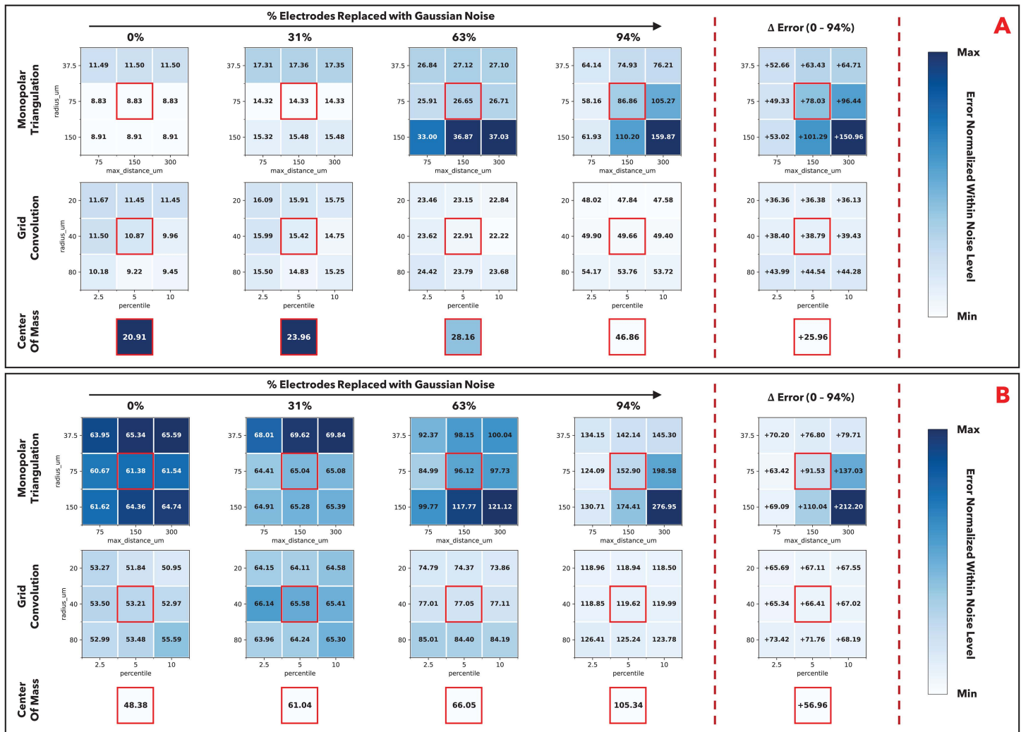
Fig 5. Impact of localization parameters on median spike localization error. For MT, we examine the parameters “radius_um” (denoting the radius around the peak channel where signal is considered in optimization) and “max_distance_um” (denoting the max distance from the COM initial estimate considered as a solution to optimization). For GC, we examine the parameters “radius_um” (similarly denoting radius around the peak channel where signal is considered in optimization) and “percentile” (denoting percentage of the best scalar products used to estimate location). For COM, the parameters have less meaningful impact on algorithm performance and so we present the median spike localization error under default parameters. Median error using the default parameters are marked in red boxes, and we examine parameters an order of two lower and higher than the default parameters. In the first four columns, we show the progression of the median localization error as electrode degradation increases, and the colors denoting magnitude of error are normalized within the individual electrode degradation level but across the three localization methods (i.e., normalized within the “column”). We additionally show the change in localization error from 0% to 94% degradation for each method and parameter set in the fifth column, to indicate how much electrode degradation impacts performance. A: Results on the simulated dataset (MEArc). B: Results on the experimental dataset (SPE-1).
