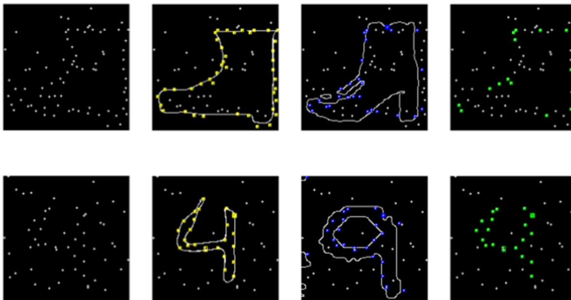
Fig 3. Quantifying solution overlap using IOU (dots). Examples from Fashion MNIST (top) and from MNIST (bottom), from left to right 1) Constellation image 2) dots covered by human drawing 3) dots covered by search algorithm drawing 4) common dots between search and human drawing. The intersection over union (dots) for this Fashion MNIST is 0.25, whereas IOU(dots) for MNIST is 0.8. The overall IOU(dots) for the whole dataset for human drawings to the corresponding search solution is 0.49 for Fashion MNIST and 0.6 for the MNIST dataset.
