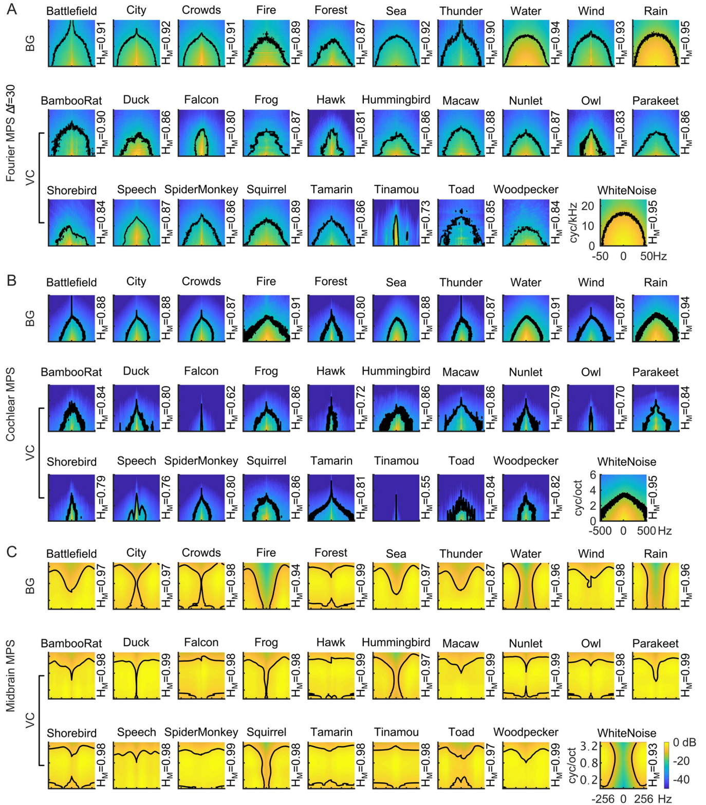
Fig 7. Modulation power spectra of natural sound ensembles including vocalizations (VC) and background sounds (BG). The modulation power spectrum is shown for the (A) Fourier-based decomposition ( \Delta f = 30 Hz), (B) cochlear model decomposition and (C) midbrain model decomposition. Whereas the Fourier MPS and cochlear model MPS overemphasize low frequency spectral and temporal modulations, the midbrain model MPS is substantially flatter. Black contours in each graph designate the MPS region accounting for 90% of the total sound power. The modulation entropy of each sound category is listed on the right side of the panel.
