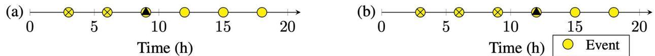
Fig 5. Yellow circles on the timeline axis indicate events. The crossed circles represent the events that are already executed. The filled triangle represents the current simulation time. After a task is executed, the simulation time jumps to the next event in the queue. An exemplary transition is shown by moving from (a) to (b).
