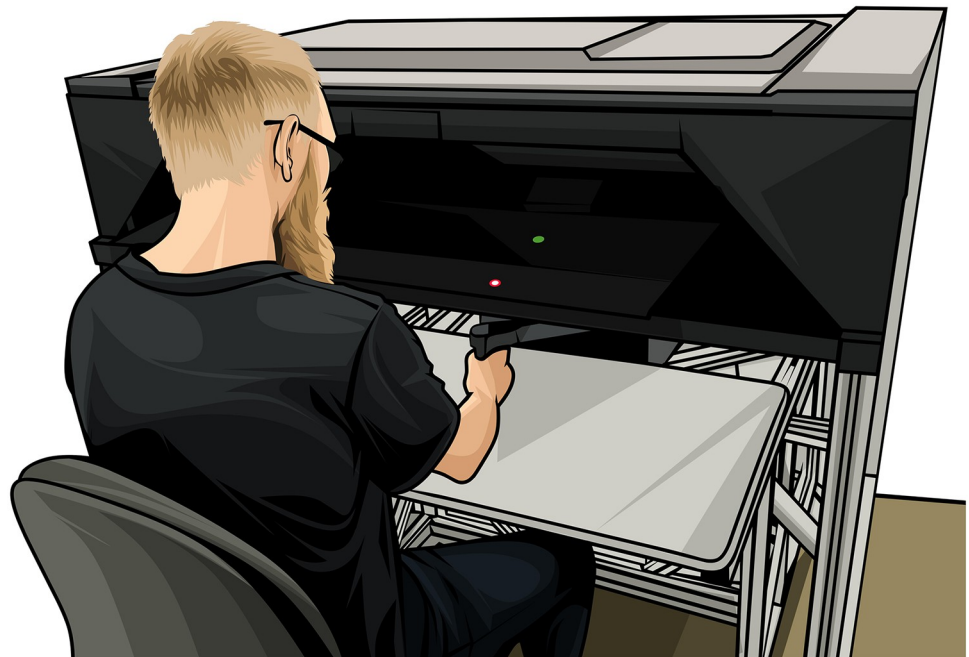
Fig 1. Experimental apparatus and task structure. Each participant made planar reaching movements while grasping the KINARM handle. A mirror system occluded vision of the hand and created the impression that the hand and visual targets were in the same plane. Red start target, green reach target, and white cursor feedback are shown.
