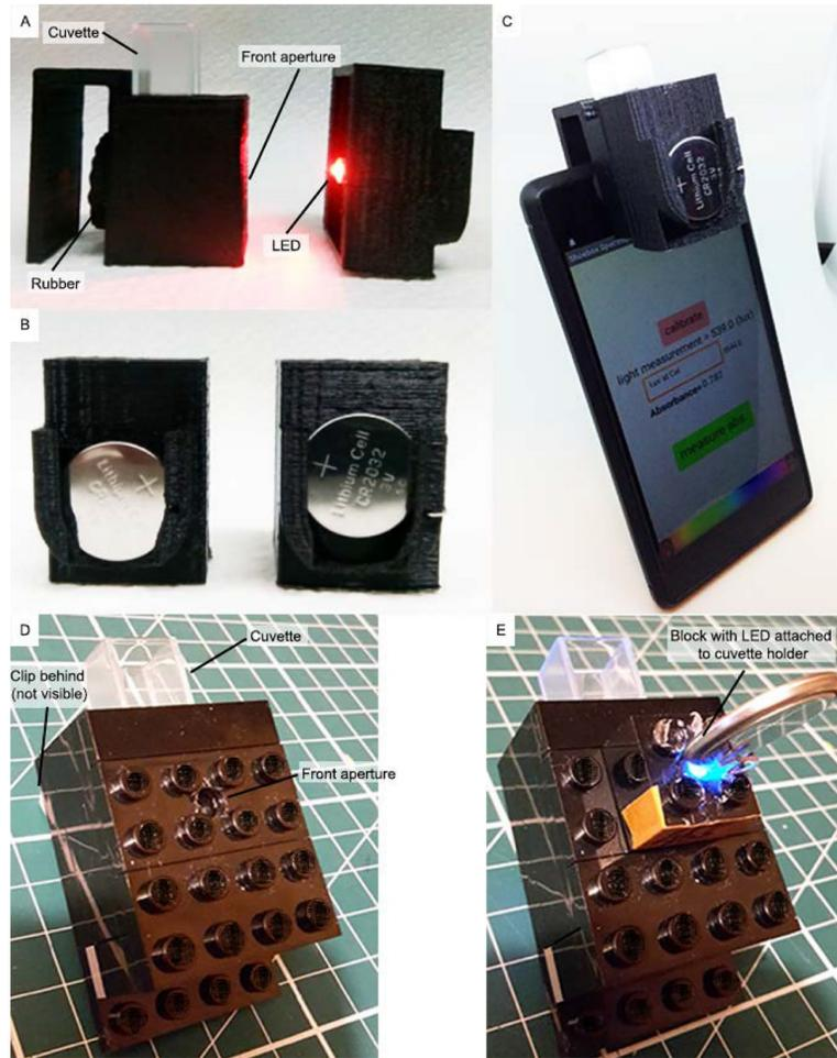
**Fig 1.** A 3D-printed version (A–C) and Lego version (D and E) of the cuvette holder. (A) Cuvette holder and interchangeable part with narrow-bandwidth LED. (B) shows the battery mechanism of the interchangeable part (pushed up for off, pushed down for on). (C) shows the holder in place. (D) shows Lego cuvette holder with front aperture, which aligns with the interchangeable Lego block with LED inserted (E). LED, light-emitting diode.
