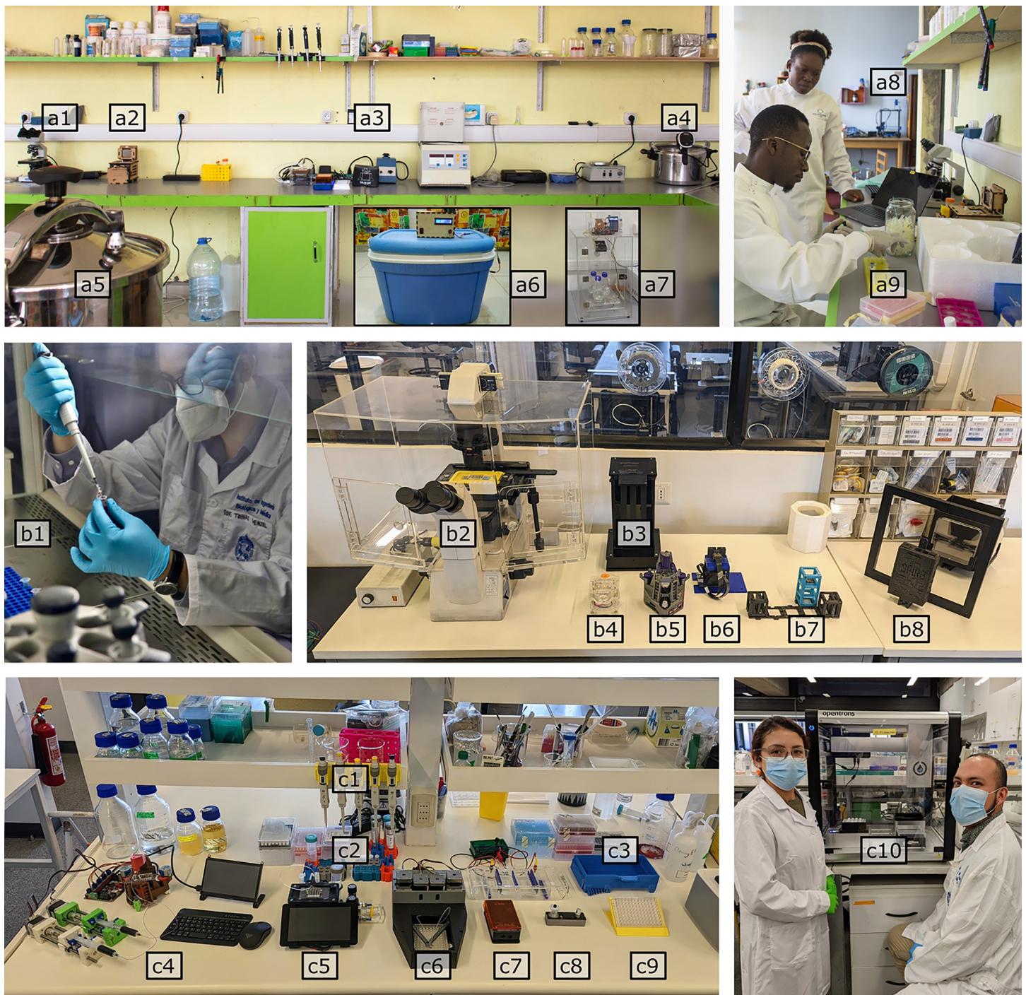
Fig 3. Examples of biology laboratories equipped with open technology. The top images show the Mboa Lab in Cameroon (source: openbioeconomy.org ) and middle and lower images show the Wenzel Lab in Chile. The following equipment is shown: basic commercial light microscope (a1), open hardware thermocycler (rebuild of OpenPCR) (a2), small commercial DNA analysis equipment (miniPCR, bluegel, vortexer, centrifuge) (a3), repurposed Sous Vide as water bath (a4), repurposed pressure cooker as autoclave (a5), self-designed open hardware incubator (a6), self-designed open hardware shaking incubator (a7), commercial open hardware 3D printer (a8), use of reagents and open enzymes (a9). Secondhand commercial laminar flow hood (b1), secondhand commercial microscope with custom enclosure and 3D-printed sample and camera adaptors (b2), open source laser-cut fluorescence plate imaging station (rebuild; [48]) (b3), open laser-cut smartphone microscope (Roachscope from Backyard Brains) (b4), open 3D-printed OpenFlexure microscope in fluorescence configuration (rebuild and star-LED fitted; [49]) (b5), 3D-printed computational microscope (rebuild with Unicorn Raspberry Pi hat) (b6), open 3D-printed holographic microscope (UC2 rebuild; [31]) (b7), open time-lapse multiple Petri plate imaging system (SPIRO rebuild in progress; [50]) (b8). Student-designed 3D-printed pipette holders with earthquake safety (c1), open 3D-printed tube racks (rebuild from Dormant Biology Lab design) (c2), 3D-printed pipette tip aligner for tip box refill (Elster rebuild) (c3), self-designed microfluidics educational workstation (Raspberry Pi-based control of 3D-printed syringe pumps and microscope) (c4), open workstation for integrated single-cell transcriptomics (RNA-seq miniDrops rebuild; [33]) (c5), open 3D-printed microscopy pipetting robot that can be mounted on a microscope (rebuild in progress; [32]) (c6), open-source gel electrophoresis set (self-designed parametric laser-cut gel chamber with open commercial IORodeo power supply and IORodeo blue LED transilluminator) (c7), open thermocycler (Gaudilab PocketPCR built from commercial set) (c8), open self-designed well-plate locator stand (c9), open commercial pipetting robot OpenTrons (c10).
