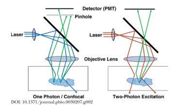
Figure 2. Effect of Scattering in Confocal Microscopy and Two-Photon Excitation Microscopy
