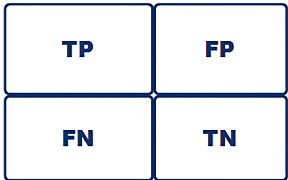
Fig 2. Classification performance metric. Confusion matrix. Made up of predicted values and actual values presented to show how many true positive predicted values, true negative predicted values, false positive predicted values and false negative predicted values were obtained by each predictive model.
