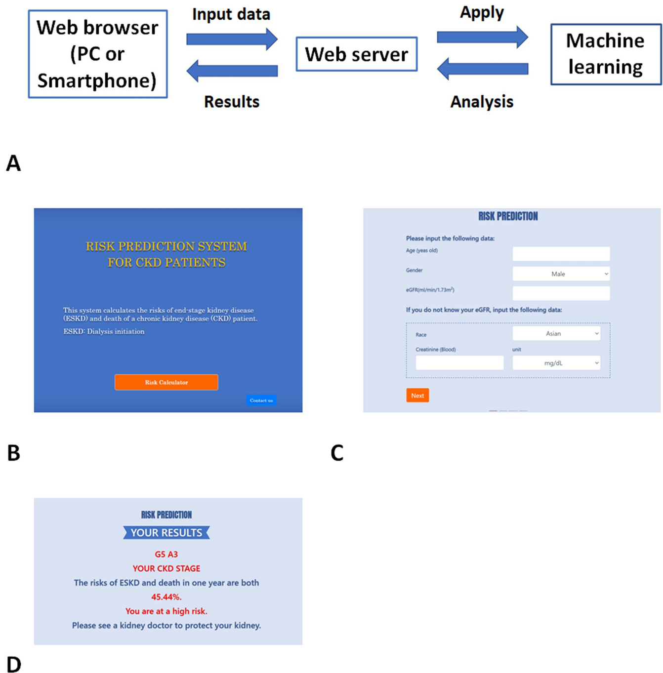
Fig 4. Images of Web pages of risk-prediction system. A. Conceptual design of the system: Patients' data are input to the machine-learning models. The results are shown on the browser. B. Start page: Go to the Web site, http://160.16.88.112:8000/ . C. Input page: Input data of a patient. D. Result page: The expected probability is shown with messages to focus the user's attention on CKD. Abbreviation: CKD, chronic kidney disease.
