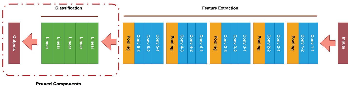
Fig 2. The VGG-16 architecture used for our experiments, with layers where sparsity techniques were applied highlighted by a red border and labeled as “pruned component”.
