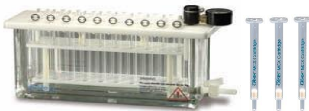
Figure 4 Solid Phase Extraction (SPE) apparatus and MCX cartridges
