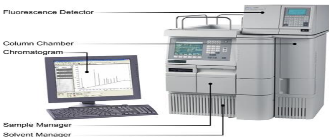
Figure 1 Typical HPLC system. Sourced from Waters (2013b)
