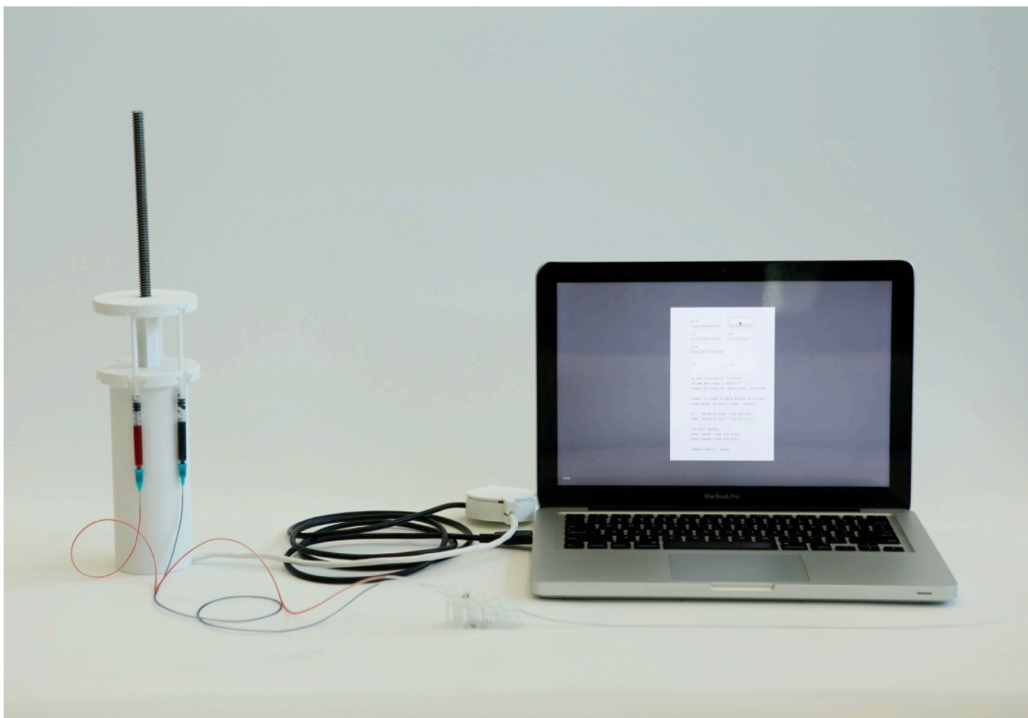
Fig. S5 | 3D printed syringe pump. A bespoke syringe pump and user interface was designed and fabricated for this experiment. The syringe pump was used to pull the two inputs through the device at 1 and 5 \mu\text{L}/\text{sec} . The syringe pump is composed of several parts ( Fig. S7 ), including 3D printed mechanical pieces, a custom designed and fabricated circuit board ( Fig. S9 ), and a software user interface ( Fig. S10 ). The CAD designs and software for the syringe pump have been made openly available. The total cost of the pump was $56.33 ( Table S2 ) and the 3D printed components can each be printed in less than 3 hours. Photo credit: Taylor Levy and Che-Wei Wang.
