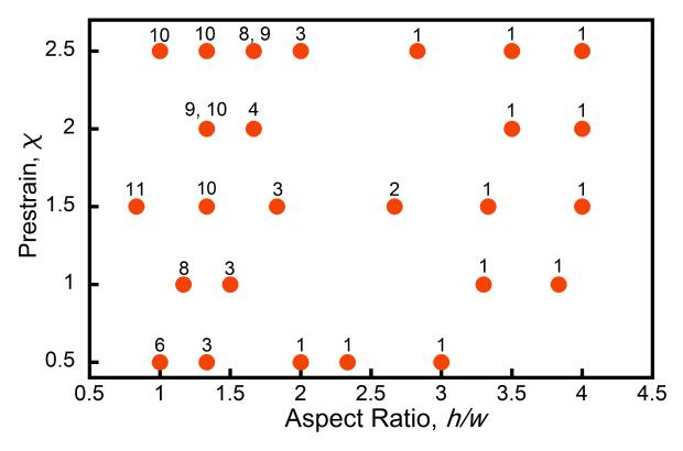
Figure S5: Phase diagram obtained when both ends of the bi-strip are clamped to prevent them from rotating. Compared to the phase diagram when the ends are free to rotate, the main difference is that helices do not form. Also, the number of perversions formed can be slightly different. For example, for h/w = 2.67 and  $\chi = 1.5$ , there is only one perversion when the ends can rotate but two perversions when they are clamped. The length, L, is 50 cm for each bi-strip.
