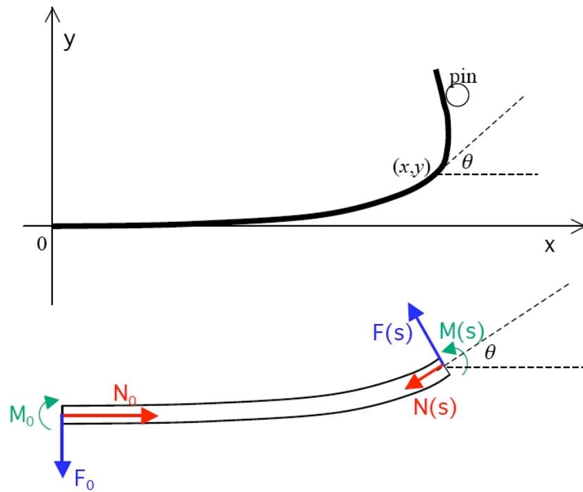
**Figure A1. Elastic beam.** Top: coordinates used in the calculation.  $\theta$  is the angle between the beam tangent vector and the  $x$ -axis. Bottom: A segment of the beam, between the origin and  $s$ , showing the forces and moments applied to the ends. Red: normal forces. Blue: shear forces. Green: bending moments. Note that the bending moment at  $s$  is defined to be positive if it produces an upward curvature.
