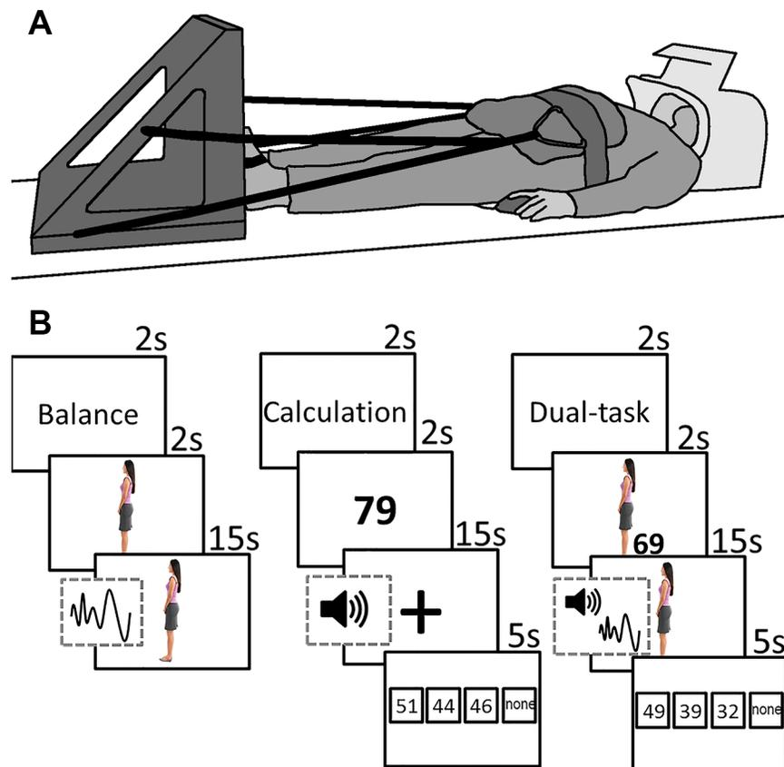
**Fig 1. A:** Illustration of experimental setup in the scanner. Participant lies supine with her feet against the force platform. **B:** Schematic of the stimuli during balance, calculation and dual-task conditions. The sine wave signifies the addition of the disturbance signal, causing the avatar to sway forward and backward. The speaker signifies the addition of beeps, which indicated the time points at which the participant had to subtract.
